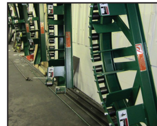
Assembled Roller Turn Rolls that will be installed in an overhead paint line
